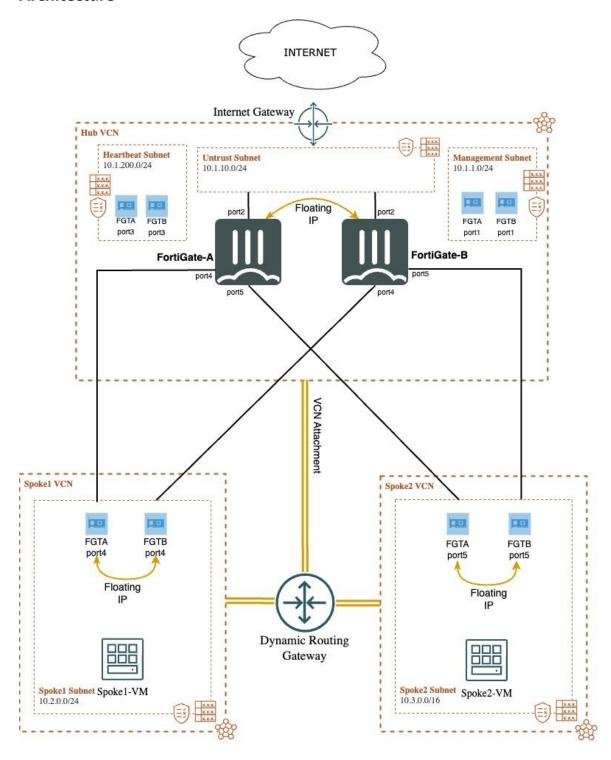
This diagram illustrates a high availability (HA) network setup using FortiGate firewalls in Oracle's C3 and PCA X9-2 platforms. It demonstrates secure and resilient communication across hub-and-spoke topology using cluster FortiGate virtual machines configured with failover and required routing.
