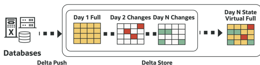
Figure 2. Zero Data Loss Recovery Appliance: Delta Push & Delta Store
